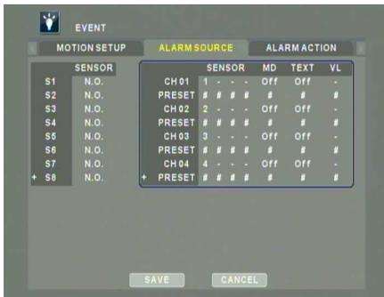
In case utilizing Alarm Inputs for alarm recording, configure the appropriate circuit type, N/O or N/C. Additionally, PTZ event preset may be configured. When an event such as alarm trigger, motion, or video loss occurs, APEX DVR sends preset command to PTZ camera.
