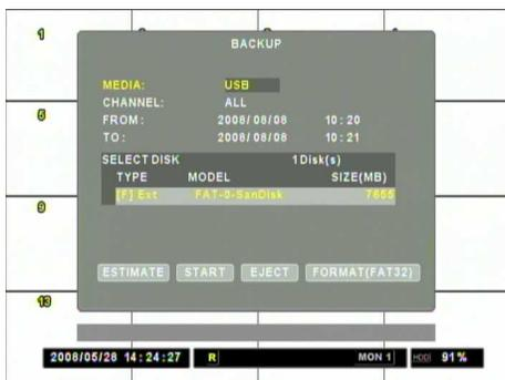
To backup as a data file, select the MEDIA as USB, then enter the desired backup range. Next, select START and press ENTER to begin. To backup specific cameras, set the Channel as CUSTOM thereafter, select the CHANNEL LIST and press the number buttons associated with the camera numbers. Please be advised that Estimate value is calculation based on all cameras.
