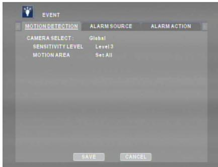
Motion grids as well as the sensitivity level can be adjusted under Motion Setup. If Camera is set as ALL, the values will be applied to all the cameras. To make individual adjustment, select Camera Select and then press the left or right arrow button to desired channel.
