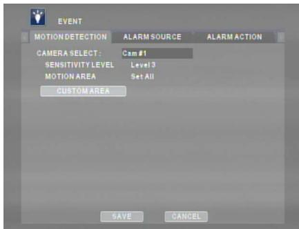
By default, all the motion grids are activated. However, to customize, select the camera then select MOTION GRIDS to display motion grid.
