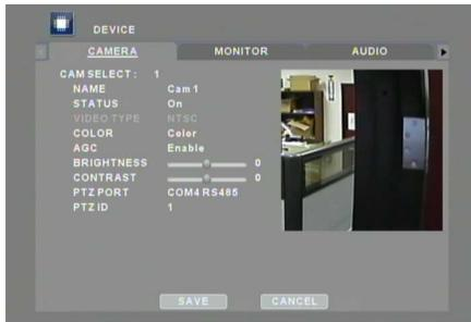
Configure the properties of cameras such as name, Camera Type (color or B/W), AGC, brightness, contrast, PTZ port, and PTZ ID.
