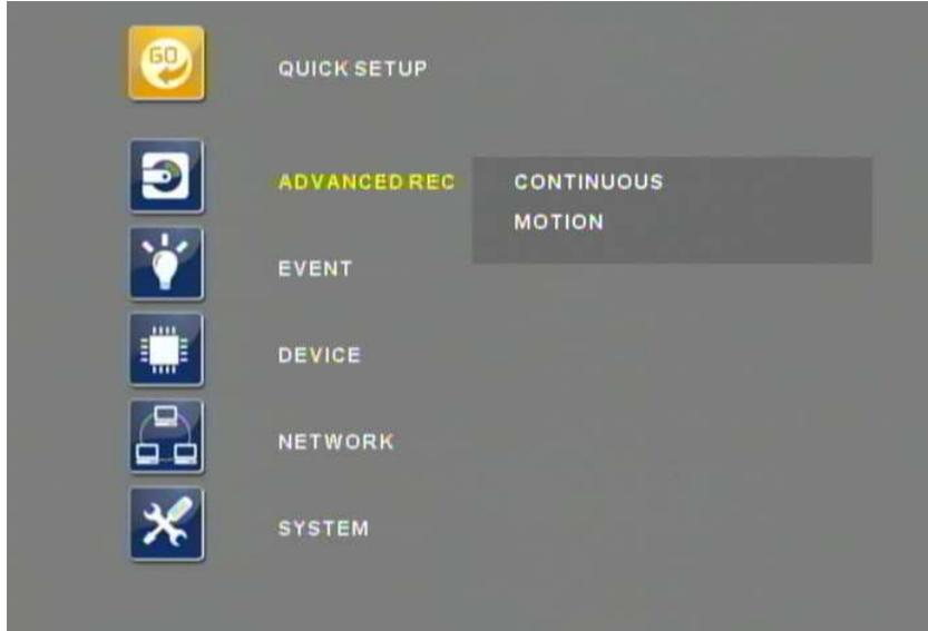
ADVANCED RECORD offers two modes, SCHEDULE ON and SCHEDULE OFF. With SCHEDULE OFF, users may set different recording parameters on a camera by camera basis. Detailed recording configuration may be set by turning on the schedule option. With the SCHEDULE ON, the APEX DVR offers more detail-oriented recording options, including BY ALARM.
