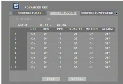
Enter the desired record setting for nighttime recording.
