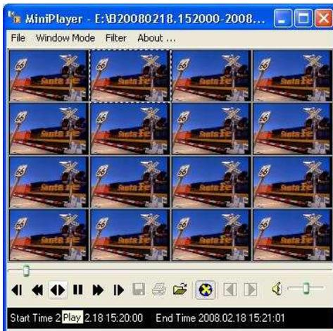
Upon Backup, the Mini Player will be copied into the optical media or USB thumb drive automatically. There is no need to install separate software to view the clips. For advanced playback options, please use NUVICO EasyNet - VMS.
