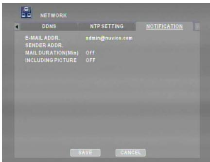
Enter user's e-mail address. The DVR will send notifications related to the system abnormalities such as HDD Fail, Alarm, Fan Fail, Password Fail, DDNS Register Fail, and Video Loss. ATTACH PICTURE option is supported when ENCODING PRIORITY is set to RECORDING.
