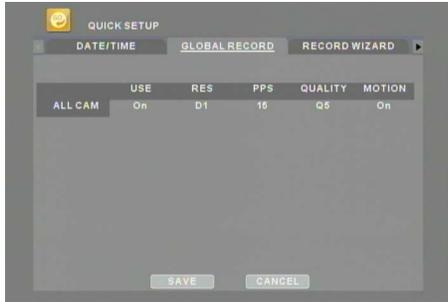
GLOBAL RECORD may be used to apply one record setting to all cameras. For resolution, D1 stands for 720 x 480, FIELD stands for 720 x 240, and CIF stands for 360 x 240. Enter the desired recording values then select SAVE to apply.
