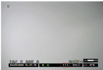
Press PTZ button to initiate PTZ function. The PTZ icon will appear on the status bar. Thereafter, use the navigation buttons, as well as Tele and Wide buttons, to control the PTZ camera. In case using NUVICO protocol, the PTZ camera menu can be accessed by pressing MENU button.
