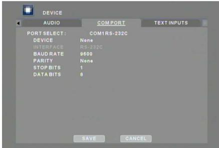
Configure devices such as PTZ cameras and Keyboard Controller that utilize COM ports. RS-232C is fixed for COM1&3 and RS-485 is fixed for COM2&4. After making physical connection, Select the appropriate device and then enter the corresponding baud rate, parity, stopbit, and databit.
