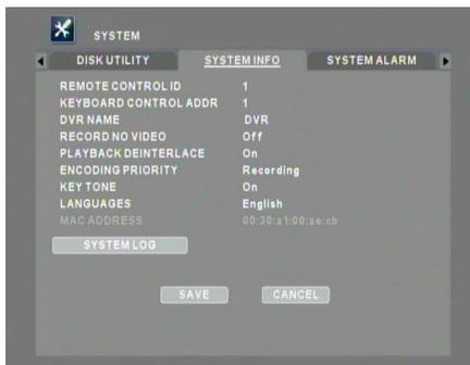
REMOTE CONTROL ID, KEYBOARD CONTROL ADDR, DVR ID, RECORD NO VIDEO, PLAYBACK DEINTERLACE, ENCODING PRIORITY (Recording/Network), and KEY TONE, can be adjusted. SYSTEM INFO also displays the Mac Address of the DVR. \*For faster streaming purpose, DVR may compensate some frames from recording when the Encoding priority is set to Network.
