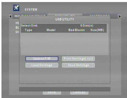
This menu allows users to update firmware and load/save settings with a USB thumb drive. Settings(.txt) option is for future implementation.
