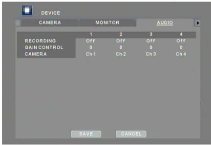
DVR allows user to synchronize audio channels with desired video channel. Also, the Audio Gain level may be adjusted.
