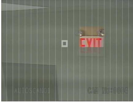
Use the combination of the enter button and the directional buttons to activate or de-activate the grids.
