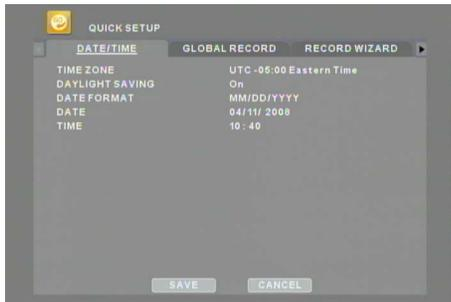
Go to the Menu then select QUICK SETUP to configure the appropriate time zone, daylight saving option, date, and time.
