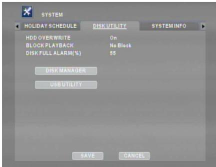
By default, the hard disk drive will overwrite from the beginning when it becomes full. BLOCK PLAYBACK and DISK FULL ALARM features can be modified, if desired.
