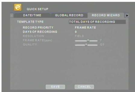
Set recording priority with FRAME RATE to maintain FRAME RATE at the maximum level. As the number of days increase, the DVR may decrease the resolution and the picture quality as compensation.
